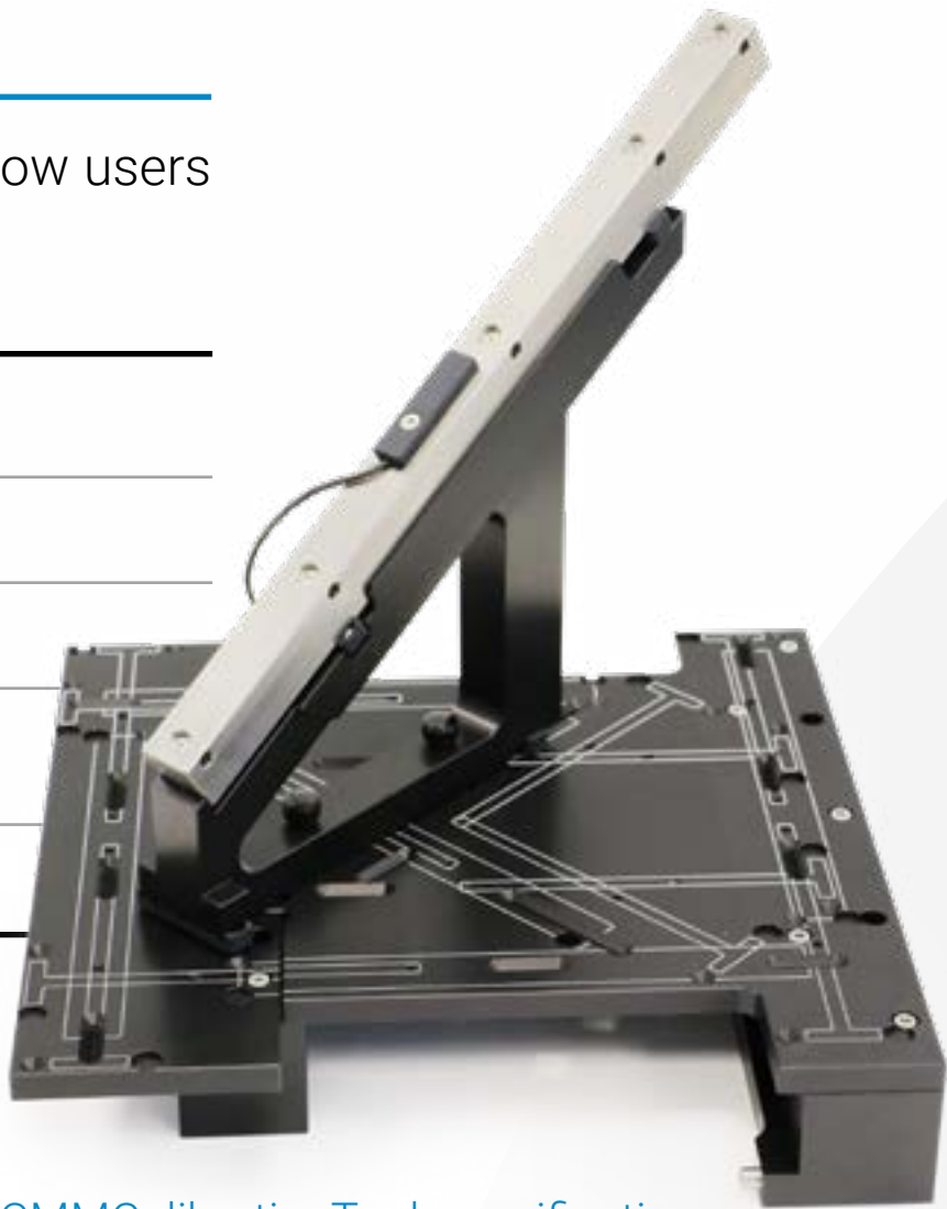
μCMMCalibrationTool – verification of larger distances based on ISO 10360-8
